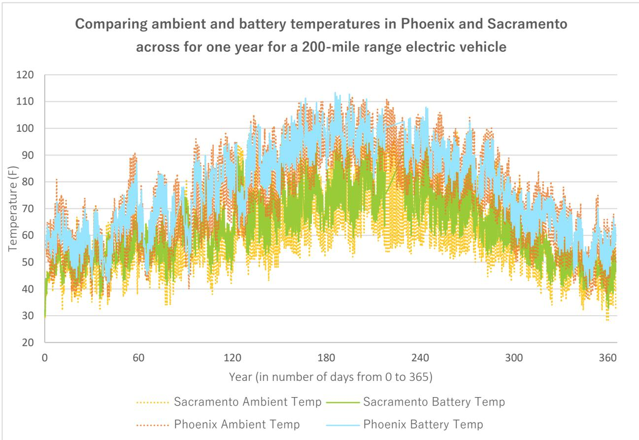
**Figure 4.** Results from BLAST-V Lite comparing for Sacramento and Phoenix ambient temperature and battery temperature for a 200-mile range ZEV with identical driving and charging patterns over one year (365 days).
