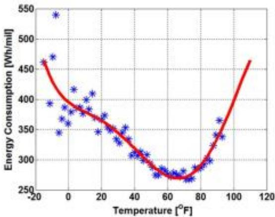
**Figure 1.** Nissan Leaf energy consumption per mile versus air temperature, using FleetCarma data.
